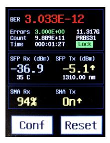
The Eye-BERT user interface consists of the main measurement screen and three configuration screens. The measurement screen is divided into three sections: the BERT area, the SFP/+ area, and the SMA/electrical area. All status and measurements are displayed on the main measurement screen; these are described in detail in the table below. Additionally there are two buttons near the bottom of the screen which are used to enter the configuration screens and reset all BERT counters.
