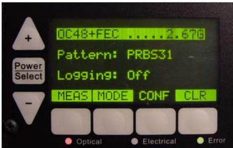
Press the “Conf” soft key and use the “Power/Select” key to highlight the desired parameter; change the setting by using the up / down buttons. When the “Meas” soft key is pressed the change will take effect.
