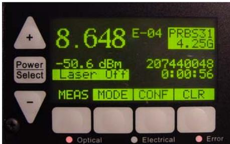
The Optical BERT measurement screen is shown to the left and displays all the associated measurement parameters. The actual bit error rate is displayed in the upper left corner with the optical input power below. The pattern and bit rate settings are displayed in the upper right corner with the actual error count and test time just below. The laser can be turned on or off by pressing the “power/select” button and is indicated below the optical power read out.
