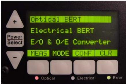
Press the “Mode” soft key and use the up / down buttons to highlight the desired mode, when the “Meas” soft key is pressed the change will take effect.
