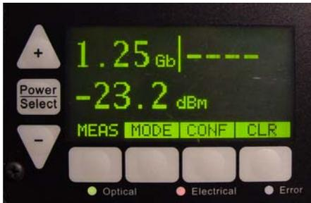
The E/O & O/E Converter measurement screen is shown to the left and displays all the associated measurement parameters. In this mode the Eye-BERT converts the optical input signal to an electrical output and the electrical input to optical output. The unit automatically searches for K28.5 symbols at the predefined data rates, and once detected, displays the bit rate, retimes the output data, and generates a recovered optical half rate clock output.
